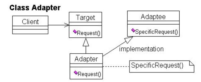
Convert the interface of a class into another interface clients expect. Adapter lets classes work together that couldn't otherwise because of incompatible interfaces.
